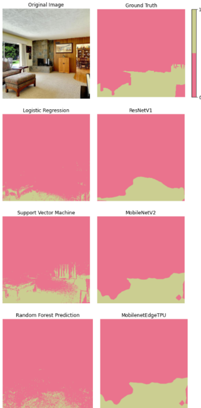
Fig. 5: Examples of predicted semantic segmentation from the six models. Instances of the non-obstacle class are represented as yellow pixels. Instances of the obstacle class are represented as pink pixels.
